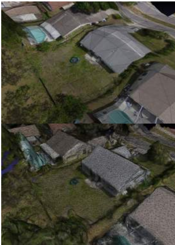
mesh-octree-depth 6 and mesh-size 10000 (top) vs. mesh-octree-depth 11 and mesh-size 1000000 (bottom)
