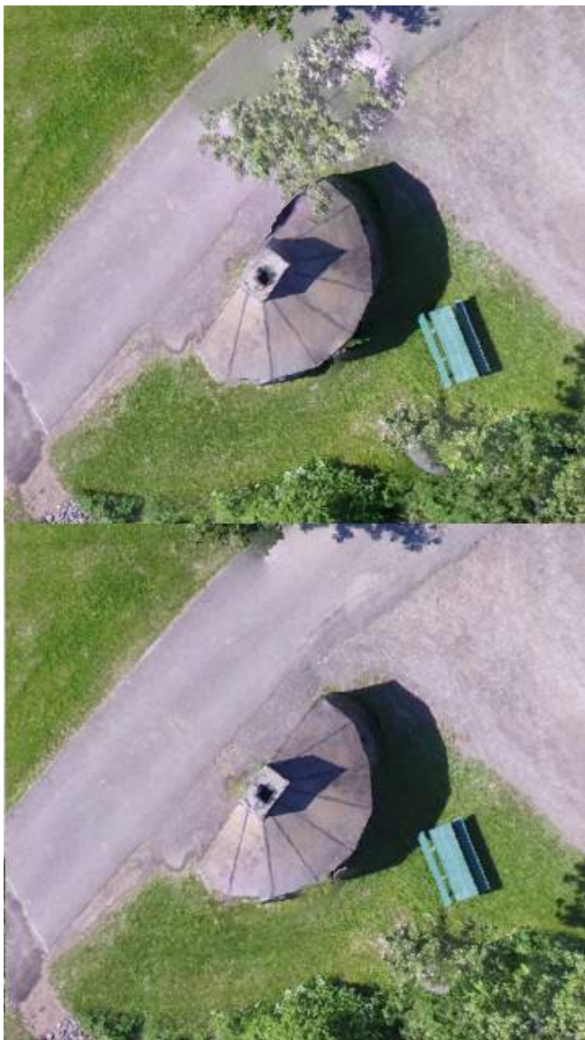
texturing-nadir-weight set to 0 (top) and 32 (bottom). Note the quality improvements near the edges of the building
