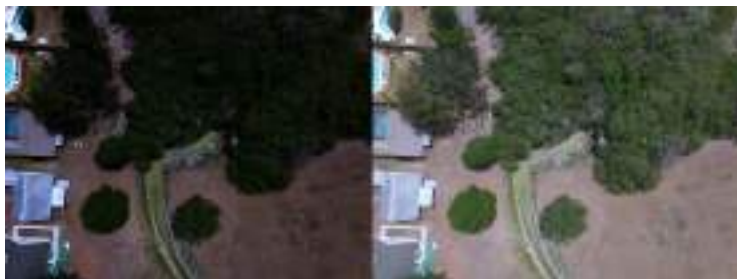
Raw input image (left), gamma corrected image (right)
