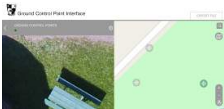
Tagging images with points using POSM GCPi
